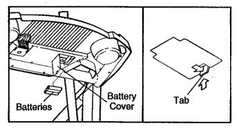
Close the battery cover, push up on the battery cover tab, and then push the tab forward as shown in the inset drawing. Make sure that the tab locks into place.
